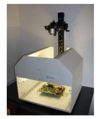
**PlatiScan LEDTest** is able to test the LED parameters **Colour** and **Intensity** with high precision.
